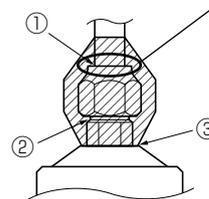
③ may become rusty as a result of coating peel-off at work using a spanner.
