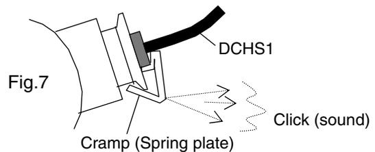
6. Connecting the compressor cables
