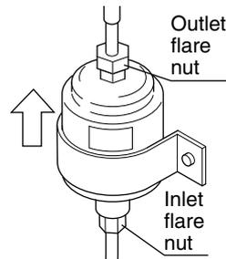
Fully apply silicon sealant to the dryer body including the flare nuts on the inlet and outlet sides.
