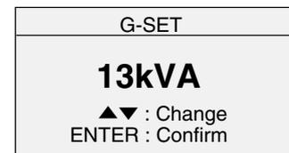
When a G-set setting has been made, the total power consumption will take priority, so that refrigeration performance may be insufficient under some conditions.
