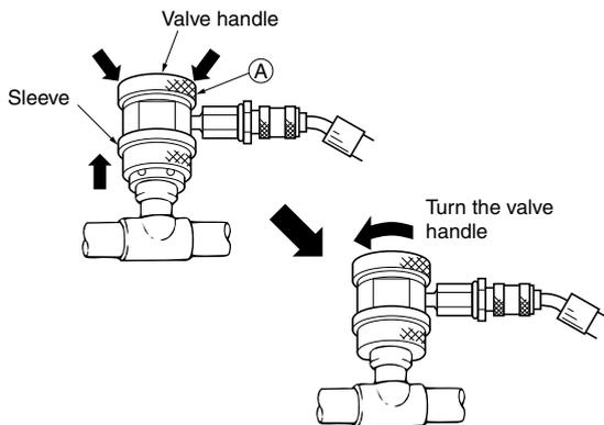
Note: Do not fully turn the valve handle clockwise. Otherwise, the push pin may be broken.
