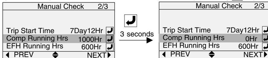
Follow the same procedure for EFH, EFL, CFH and CFL running hrs.
