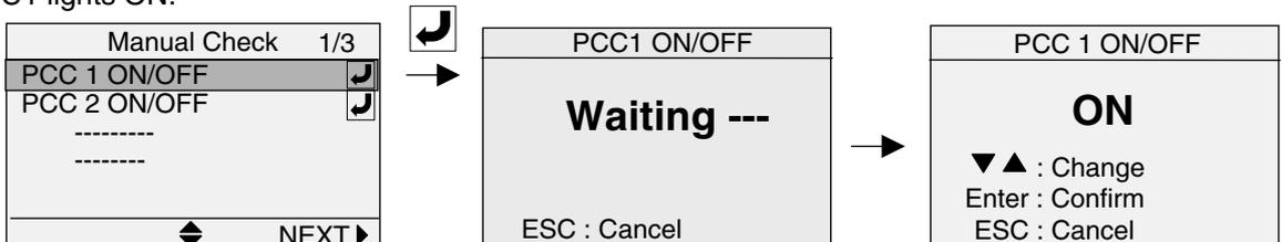
Follow the same procedure for other magnetic contactor or solenoid valve ON/OFF check.
