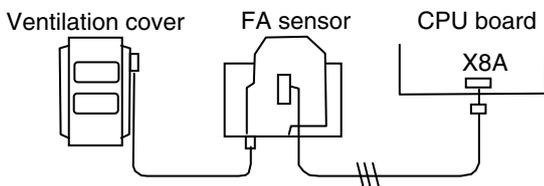
Either "Ventilator with insect screen" or "Ventilator without insect screen" is set for the unit installed with FA sensor at factory referring to ※12 Configuration Set in paragraph 2.3.
