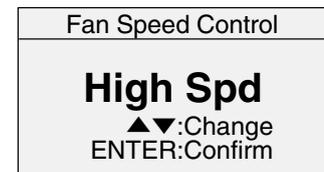
AUTO : During chilled operation, the evaporator fan runs at high speed/low speed.
