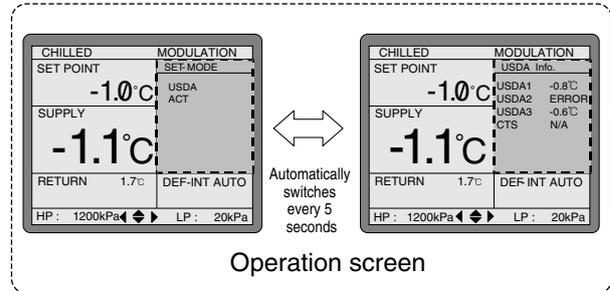
When the or key is pressed, the ACT setting status and the current operating status can be checked.
