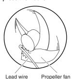
Cautions in mounting the motor Be sure to fix the motor lead wire with a clamp. Not heeding this caution will cause the entanglement of the lead wire around the fan, which will result in damage to the fan.
