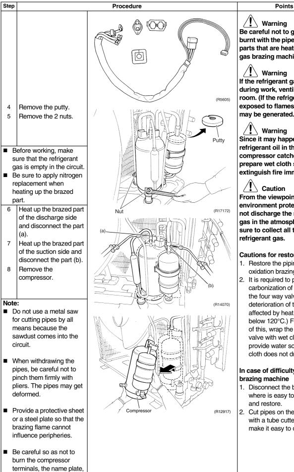
Warning Be careful not to get yourself burnt with the pipes and other parts that are heated by the gas brazing machine.
