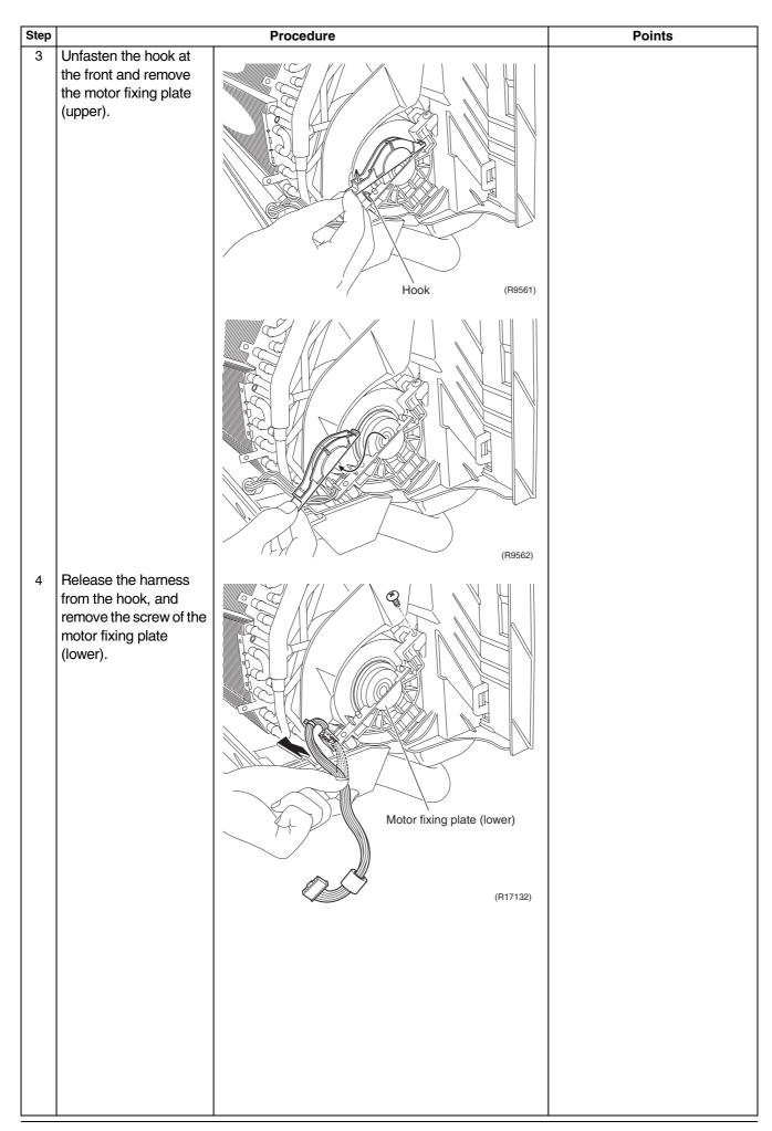
Removal of Fan Motor Si041057
