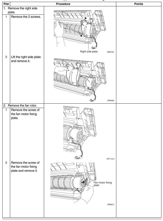
Si041057 Removal of Fan Rotor
