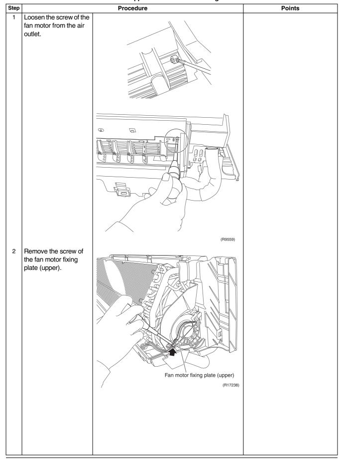
Si041057 Removal of Fan Motor
