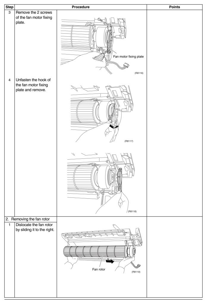
Removal of Fan Rotor Si04-953
