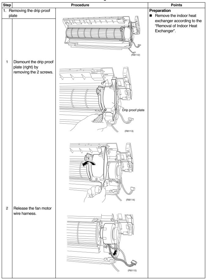
Si04-953 Removal of Fan Rotor
