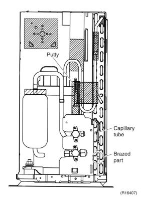
Do not use a metal saw for cutting pipes by all means because the sawdust comes into the circuit.
